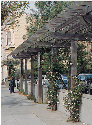
Figure 3.D.59: A sidewalk is buffered from an adjacent parking lot by an attractively landscaped wall and overhead trellis.
