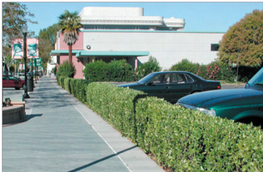
Figure 3.D.60: A hedge buffers a sidewalk from adjacent parked cars. In the evening, the hedge can prevent headlights from shining on pedestrians.
